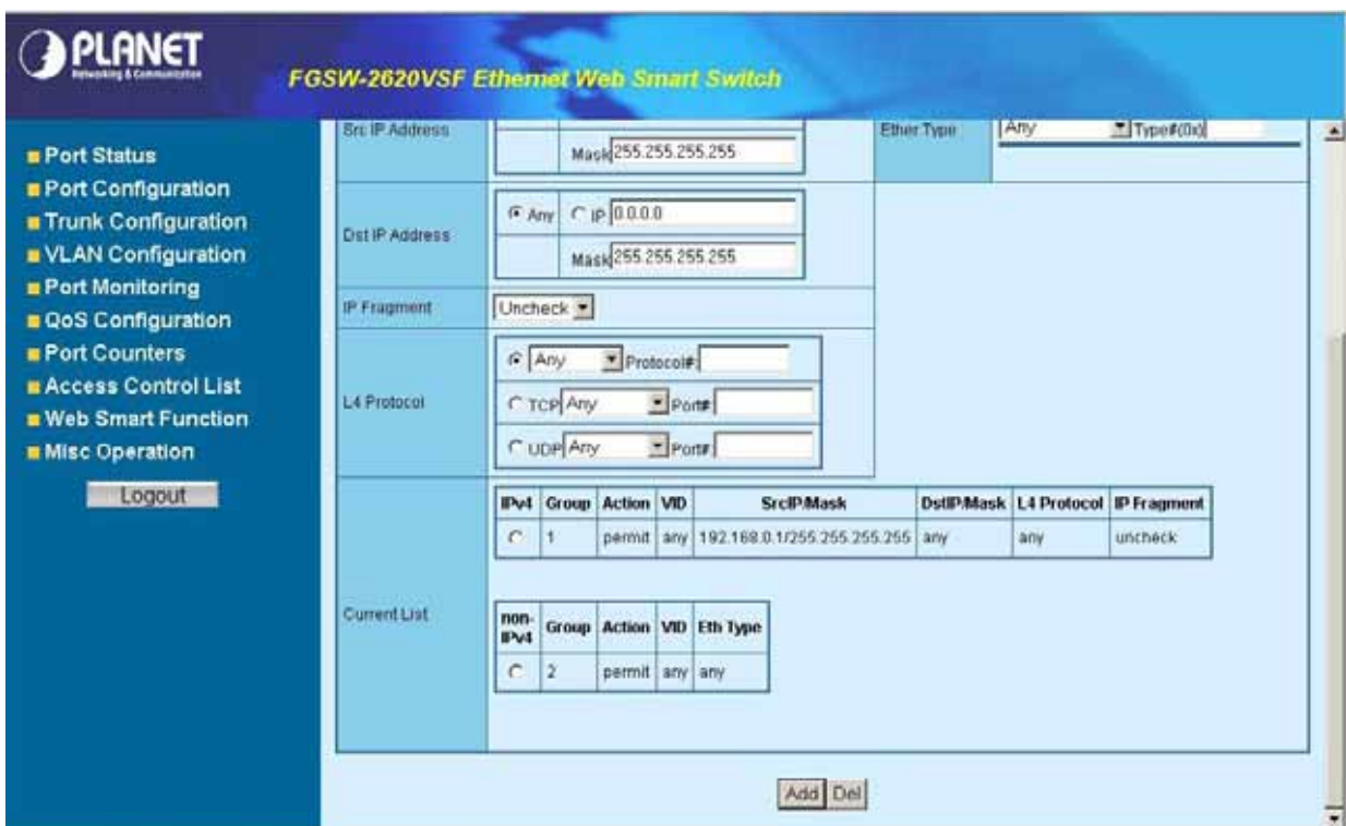
Figure 4-43 Access Control List (ACL) Web Page screen
